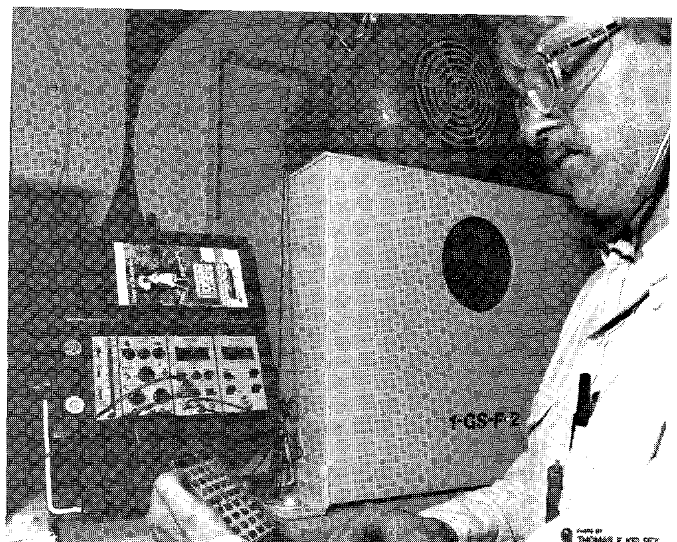
Fig. 6. Using the Type 3537 Portable Tracking Balancing Set to balance a gland steam fan
